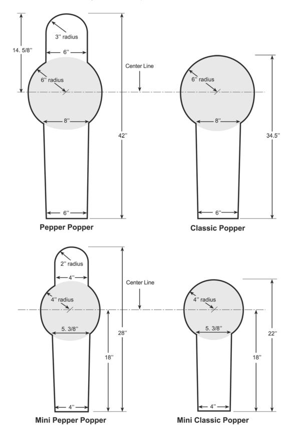
The calibration zone for each target is indicated by the shaded area.
